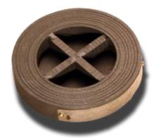
of high purity graphite impregnated with phenolic resins in order to make the product non porous Opening is total but with fragmentation. Vacuum support is required for rupture pressures below 1.7 barg. At higher calibrations the disc is selfsupporting.
